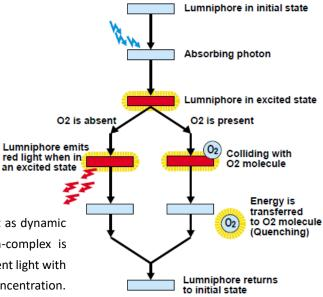
Sensor measurements are based on selected substances that can act as dynamic fluorescence quenchers. For example, for oxygen, if a ruthenium-complex is illuminated with a blue LED it is excited and emits back a red luminescent light with an intensity, or lifetime, which directly depends on the oxygen concentration. Lifetime based measurements are superior for both long-term (no drift) and fast response applications.
